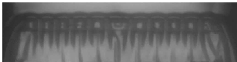
Fig. 7. Rivulet structures (H2, 25% ethyl-alcohol solution).
